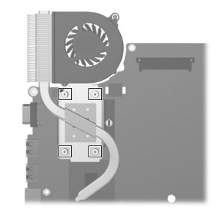
Where used: 4 captive screws that secure the heat sink to the system board
